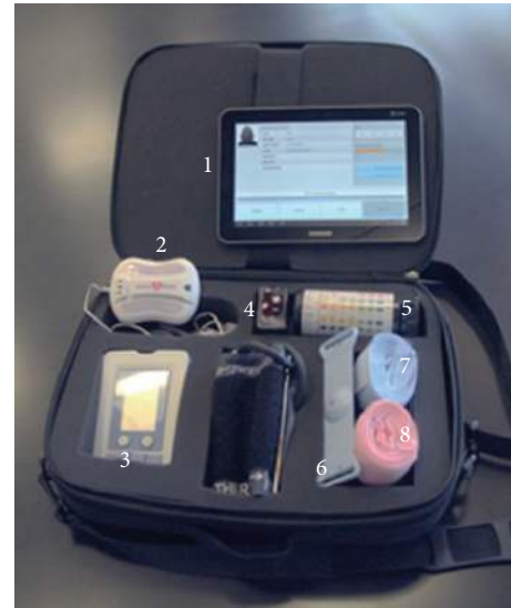
FIGURE 1: MiBebe fetal remote monitoring kit prototype technology with components as deployed in YUC, Mexico: (1) tablet/phone with fetal monitoring app; (2) fetal monitoring central unit; (3) FORA (blood pressure and glucometer); (4) pulse oximeter; (5) urine strips; (6) Toco; (7) elastic strap for central unit; (8) elastic strap for Toco.
